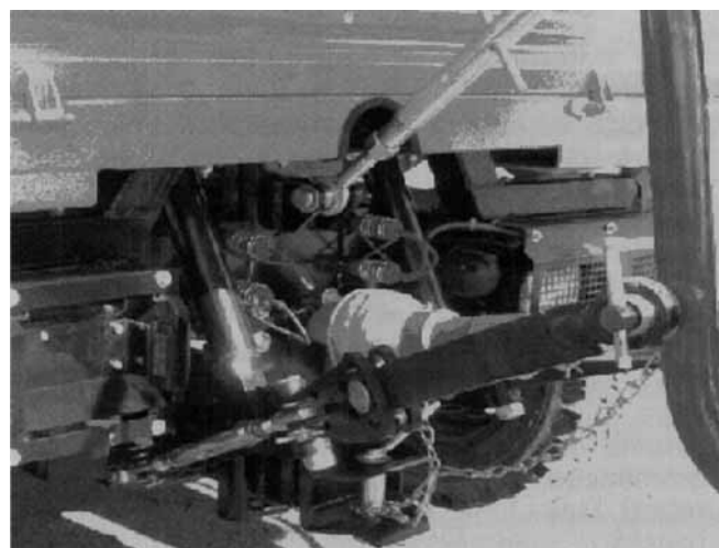
Figure 3 Photograph of rear of vehicle showing PTO shaft and hydraulic transmission.
